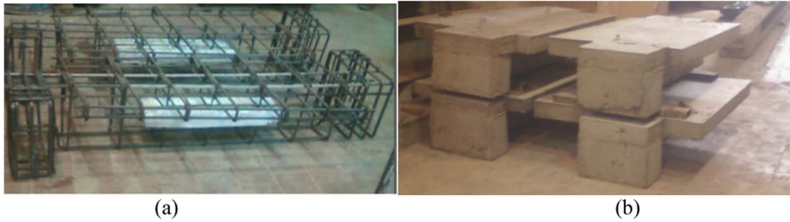
Fig. 2. Test specimens (a) reinforcement and (b) after casting.
